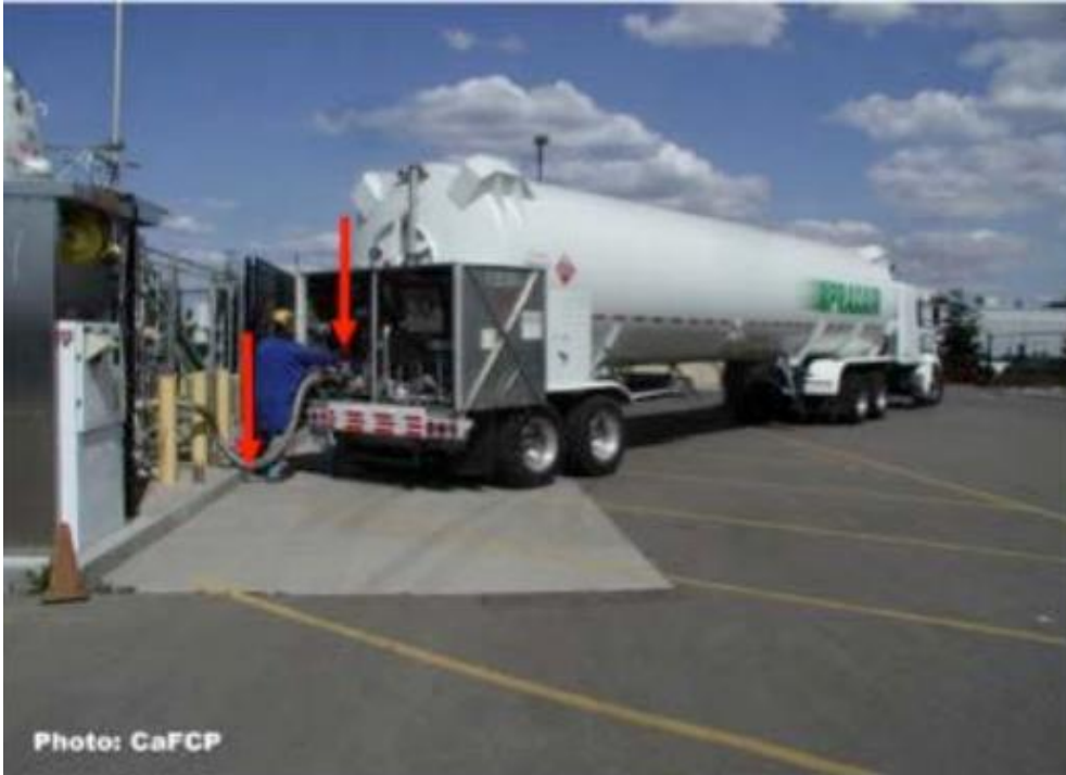
Figure 16: Liquid hydrogen transportation in insulated tank.
