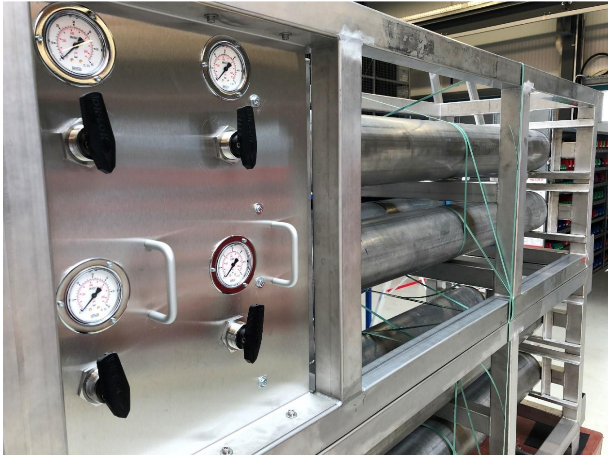
Figure 9: GKN Powder Metallurgy's storage module consists of eight separately controlled storage tanks and can store 133 kWh electric power [5].
