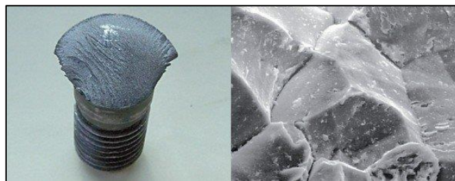
Figure 3. Bolt and Fracture Surface
